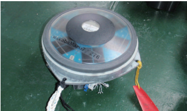
Sonar satellite buoy attachment for smart fishing buoys and other FADs to prevent outflow of fishing gear
